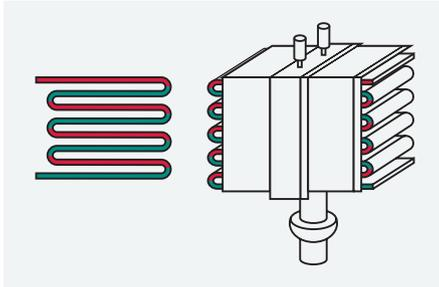
The measure of this effect is called the thermoelectric- or Seebeck- coefficient. For most conducting materials this coefficient is rather low, only few semiconductors possess rather high coefficients. Since the voltage of a single thermoelectric cell is very low, lots of such cells arranged in a series connection achieve a larger signal, making a "pile" of thermo-elements.
