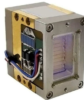
Fig. 1 Image of the High Power Diode Laser monolithic stack with 3kW laser power and pulses in the nanoseconds region. On the left side of the stack the electronics to control the short pulses can be seen.
